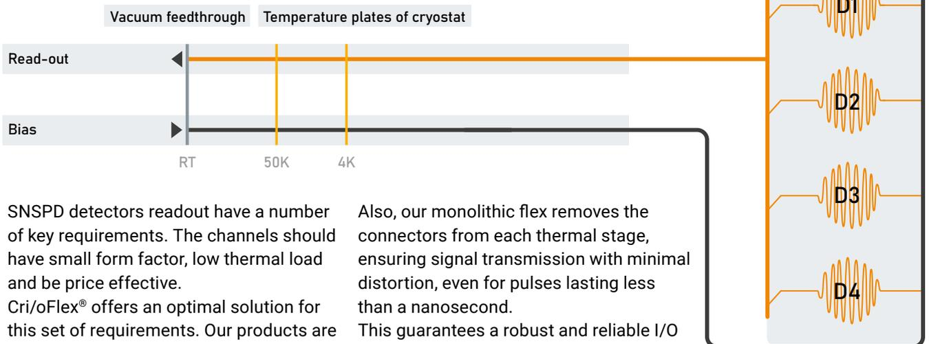
SNSPD detectors readout have a number of key requirements. The channels should have small form factor, low thermal load and be price effective. Cri/oFlex® offers an optimal solution for this set of requirements. Our products are engineered for small form factor and low heatload per channel.
