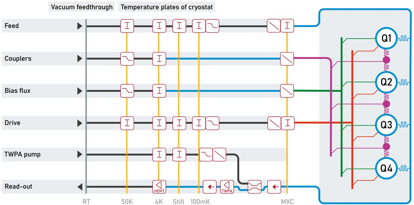
Wiring superconducting qubits poses two main challenges. First, due to an increase in qubit count, the sheer number of channels goes up, requiring many cables with a small form factor. Secondly, the qubits require different types of signals and are very sensitive.
