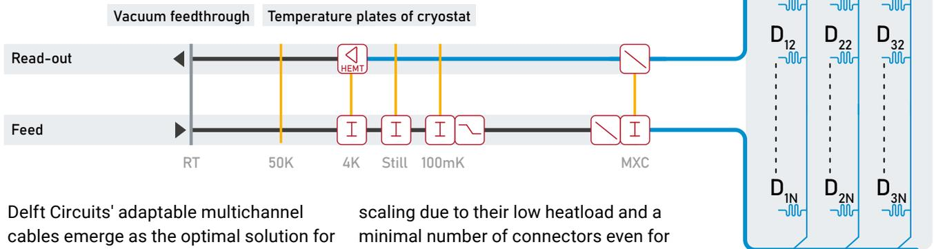
Delft Circuits' adaptable multichannel cables emerge as the optimal solution for detector arrays in astrophysics, whether deployed on the ground or in-flight. Designed with flexibility and low weight in mind, our cables enable seamless
