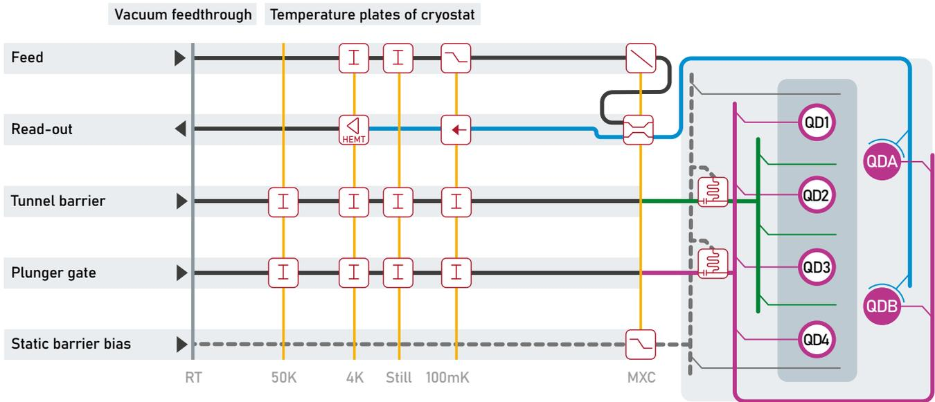
Solid-state spin quantum processors face a number of wiring challenges. Firstly, processor housings (inside magnets) have limited space, demanding small form factor interconnects for large amounts of wiring. Secondly, the quantum dot-based processors are sensitive to electrostatic noise. Our rugged flexes prevent vibration induced electric noises, overcoming
