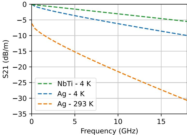
Indication of loss based on measured data
