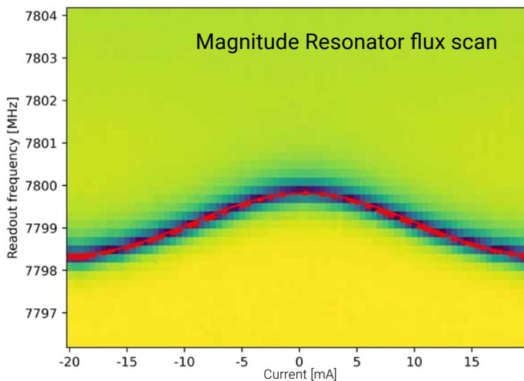
By adjusting the flux current it was possible to reach the expected sweet-spots for all qubits. When the optimal flux was chosen a Rabi scan was successfully performed.
