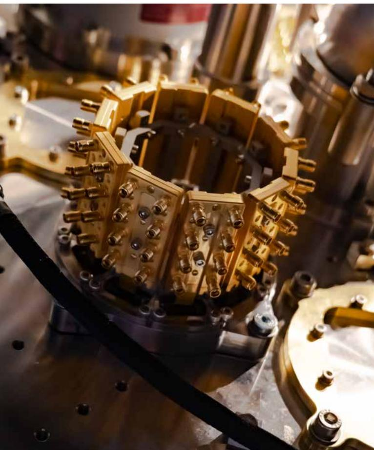
These results show that the multichannel Cri/oFlex® platform does not limit the coherence of the transmon qubits below a value of  $60 \mu\text{s}$  and can be used as an I/O platform with high scalability potential.
