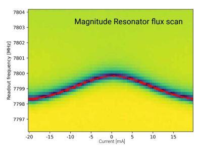
By adjusting the flux current it was possible to reach the expected sweet-spots for all qubits. When the optimal flux was chosen a Rabi scan was successfully performed.
