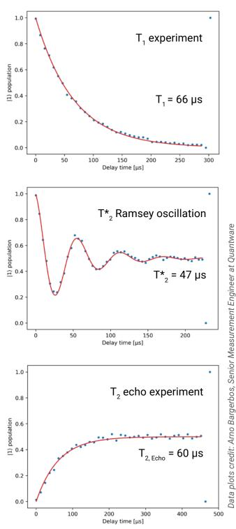
These results show that the multichannel Cri/oFlex<sup>®</sup> platform does not limit the coherence of the transmon qubits below a value of 60 µs and can be used as an I/O platform with high scalability potential.
