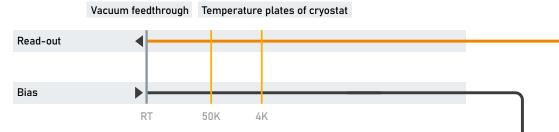
SNSPD detectors readout have a number of key requirements. The channels should have small form factor, low thermal load and be price effective.
