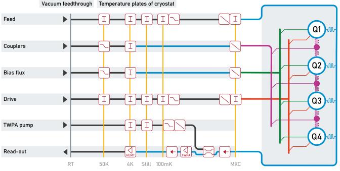
Wiring superconducting qubits poses two main challenges. First, due to an increase in qubit count, the sheer number of channels goes up, requiring many cables with a small form factor.
